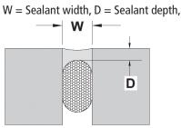
EXPANSION JOINTS - The minimum width and depth of any sealant application should be 1/4 in. x 1/4 in. (6mm x 6mm).
